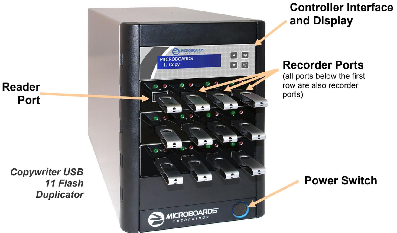
The Copywriter Flash Duplicator consists of a reader port; 7, 11, or 15 flash drive ports; and Controller module.
