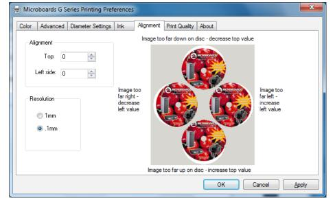
These settings will change the size of the top and left margins, respectively. Decreasing the values will move the image up or to the left, increasing will adjust down or to the right.
