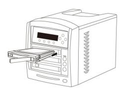
a. Securely lock the trays into each bay by sliding the tray into the bay firmly and completely.
