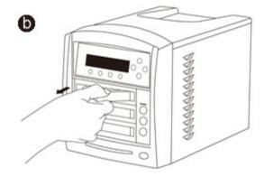
3. Insert your hard drives (both source and target) into the Hard Drive Trays.
